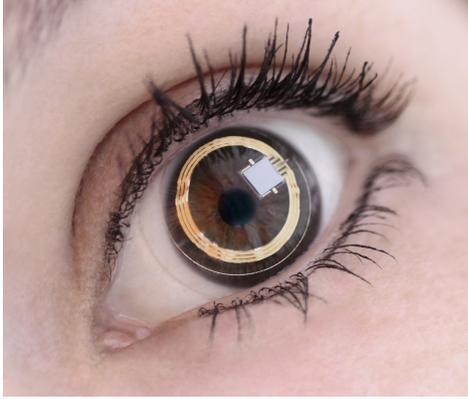
Figure 1. The contact lens sensor Triggerfish<sup>®</sup> set up in the eye.
