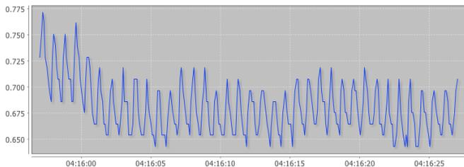
Figure 6. Example of burst captured during a sleep period. The ocular pulse, caused by the beating heart, is visible within the IOP recorded signal.
