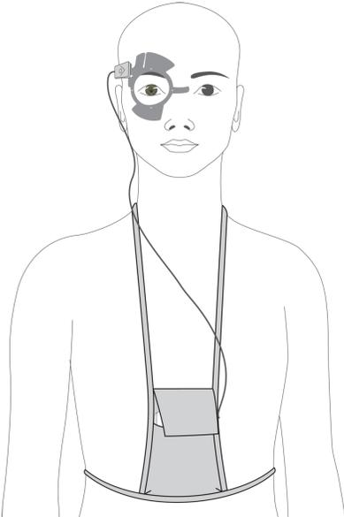
Figure 3. The Triggerfish® full equipment is composed of the contact lens sensor, the adhesive antenna and the wearable recorder.
