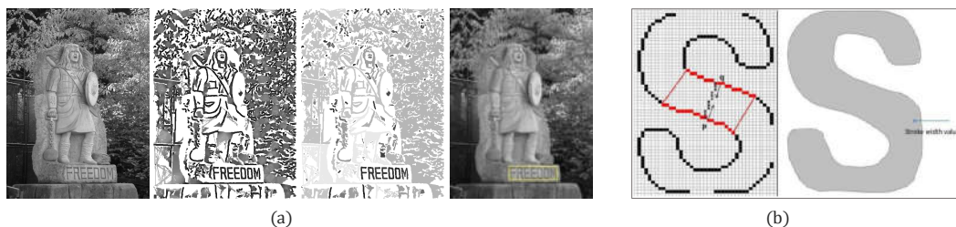
Figure 2.9: Stroke Width Transform. (a) Scene text detection examples from Epshtein’s work [EOW10]. (b) Example of SWT computation [YT12].
