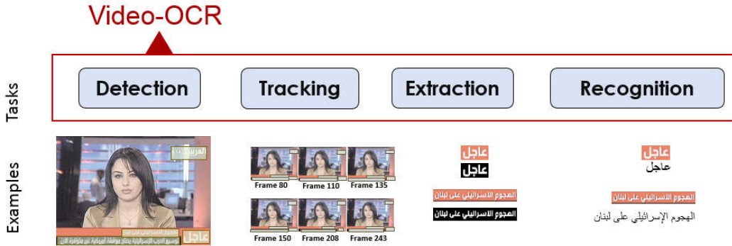
Figure 2.2: Main steps of a Video OCR system
