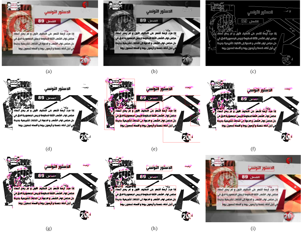
Figure 4.14: Detection process of fully heuristic-based system. (a) Input frame, (b) Gray-scale (c) Canny edge detection (d) SWT Map, (e) CC extraction (f) CCs after geometrical filtering (g) Diacritic merging (h) Textline construction (i) Refinement step and output result.
