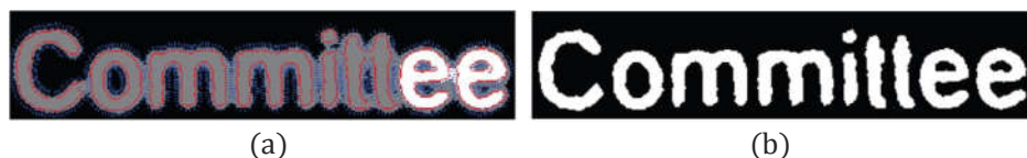
Figure 2.4: Edge-enhanced MSER, from [CTS + 11]. (a) Detected MSER for blurred text. Canny edges are shown in red lines, and blue arrows indicate gradient directions. (b) MSER after pruning along the gradient.
