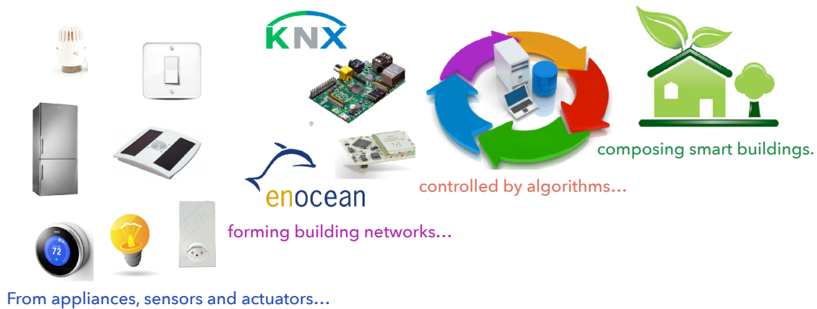
Figure 1.1: A couple of stages are required until energy savings and comfort improvement can be obtained in Smart Buildings. Control algorithms rely on functionalities offered by building networks themselves composed of smart things. They range from home appliances to sensors and actuators.
