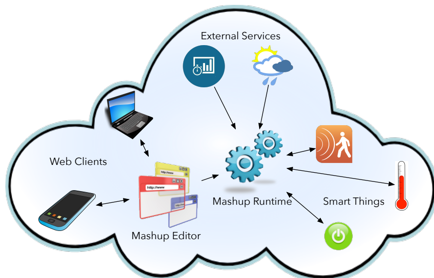
Figure 4.46: Platform overview of the mashup solution. Any kind of smart thing semantically describing its capabilities as well as external services can be used to define control scenarios.
