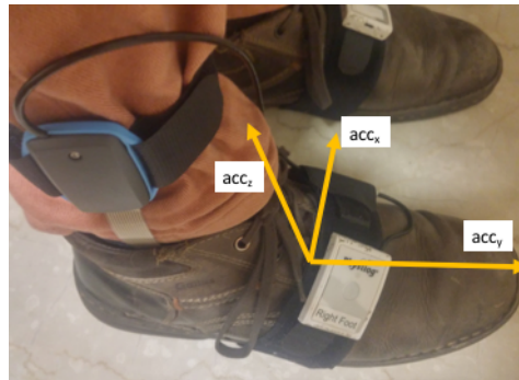
Fig. 1. Instrumented shoe setup with axes orientation
