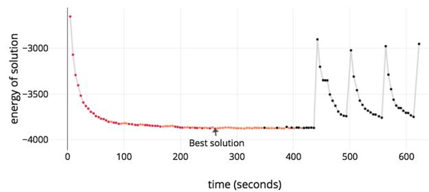
**Fig. 2** An example event showing the convergence towards the solution in each `qbsolv` loop. The algorithm occasionally jumps away from the current best solution which is an intended feature to avoid local minima
