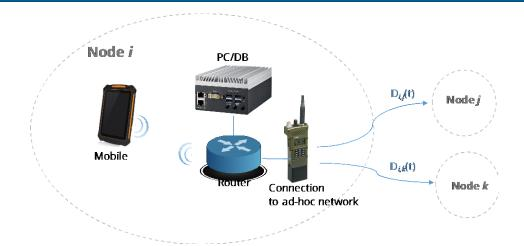
Armasuisse will test a new mobile tactical network based on wireless communications working with VHF/UHF imposing new challenges for mission critical applications. Every node in the network (see figure above) should be able to communicate at the application layer to all other nodes through an ad-hoc network. The end user will use these applications via a smartphone. Three applications will be developed: Messaging, Blue Force Tracking and Red Force Tracking.
