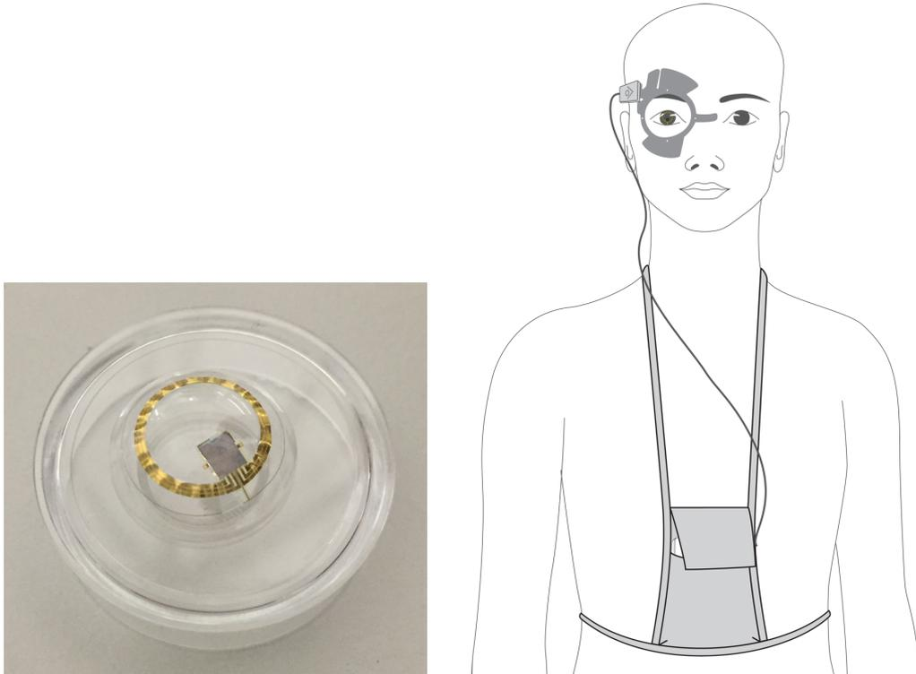
**Figure 4.3:** The Triggerfish<sup>®</sup> full equipment is composed of the contact lens sensor, an adhesive antenna and the wearable recorder [image used with permission of Sensimed SA].
