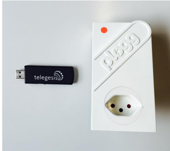
**Figure 3.10:** The *PLOGG* sensor and the *Telegesis* ZigBee transceiver (USB dongle).
