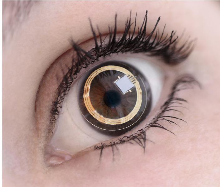
**Figure 4.2:** The contact lens sensor Triggerfish<sup>®</sup> set up in the eye [image used with permission of Sensimed SA].
