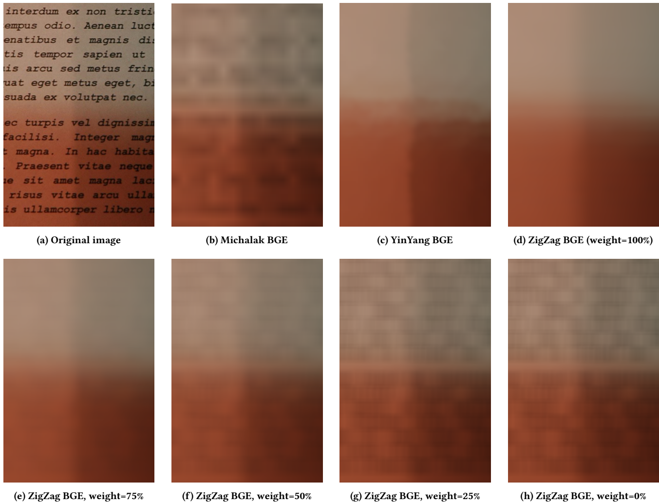
Figure 2: Comparison of background estimation (BGE) algorithms: (a) original image, (b) Michalak, (c) YinYang, and (d) ZigZag, from least to most accurate. Images (e), (f), (g), and (h) show the effect of the mean weight parameter on ZigZag’s BGE accuracy.
